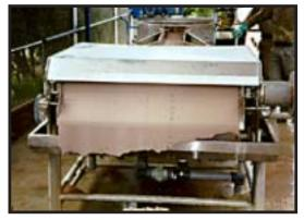
1.0 Meter Belt Press System in operation.
