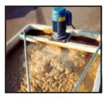
A thick layer of solids floating on the surface prior to discharge.
