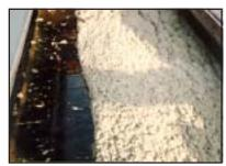
Sludge being discharged into a screw conveyor.
