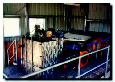
Fully automated 1.5 meter, stainless steel, skid mounted belt press
