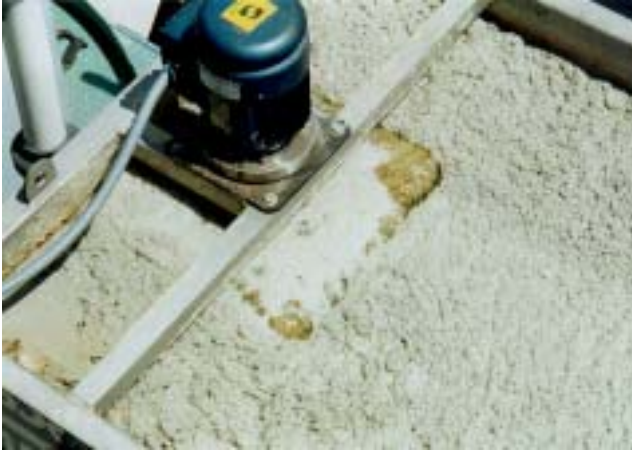
HydroCal's Cavitation Aerator injects microbubbles directly into the wastewater to make the solids rise.
