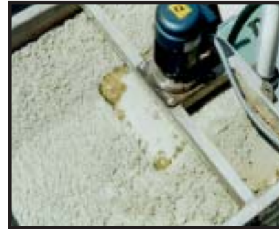
CAF in operation at a rendering plant shows the sludge layer created by the aeration bubbles.
